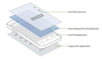
SmartTiles: A Layered Approach — Because SmartTiles are located 'above' the application layer, this allows you to position components anywhere on the screen without interfering with text fields, labels, keyboards or other critical application elements.
